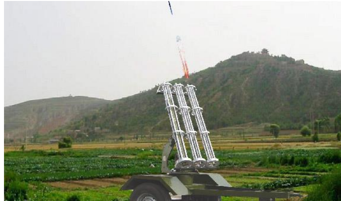
RYI-6300 model rain-inducing rockets were used in Tuv and Ömnögovi provinces in 2006-2007
