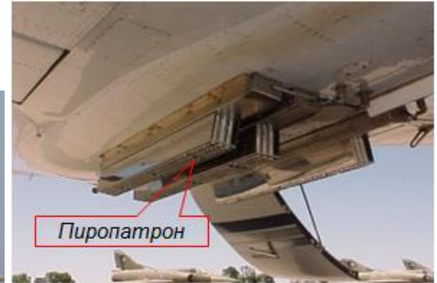
Reagent (Agl) fixed with aircraft.
